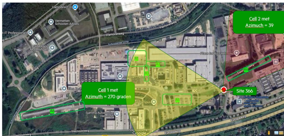
Figure 16: Radio site at Helmond automotive campus with two cells in the lowest position in the tower.
