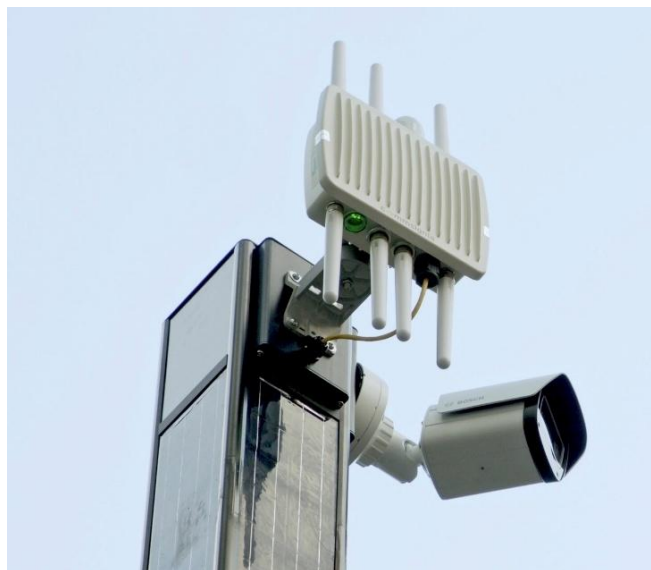
Figure 21: Commsignia RSU with smart camera.
