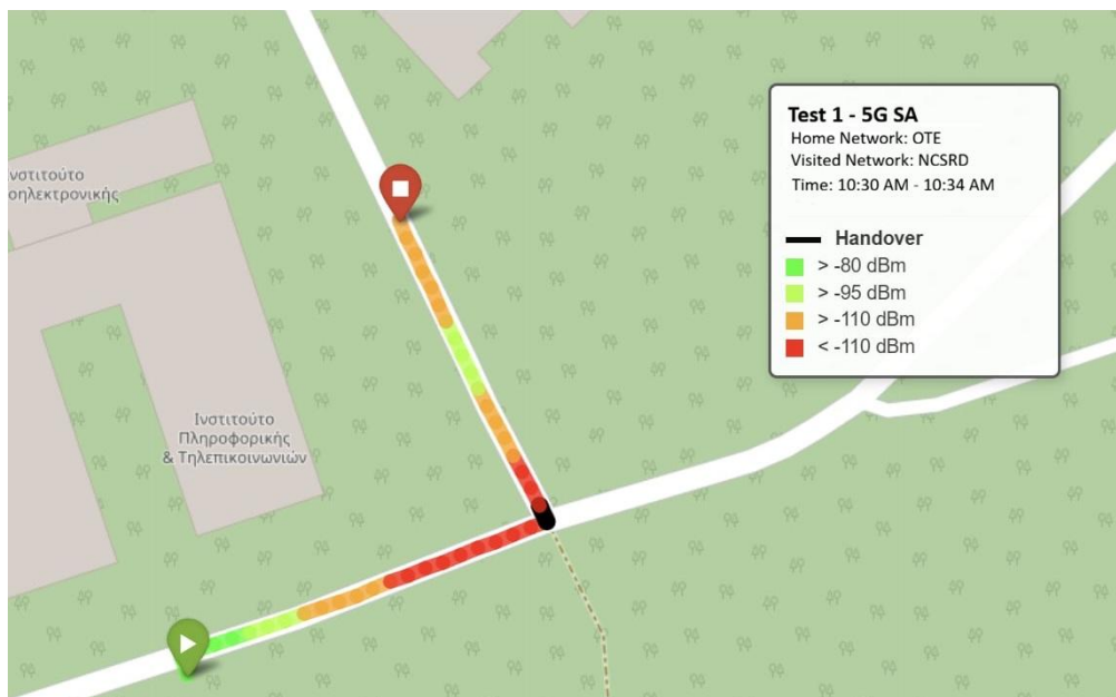
Figure 37: 5G Standalone (SA) signal-strength heatmap in the Greek trial site.
