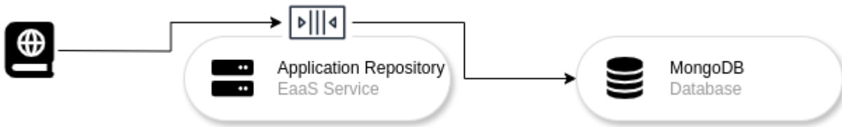
Figure 32 – Upload the package (shown on the left) by using a buffer in the Application Repository, which then writes the data to MongoDB for persistent storage.
